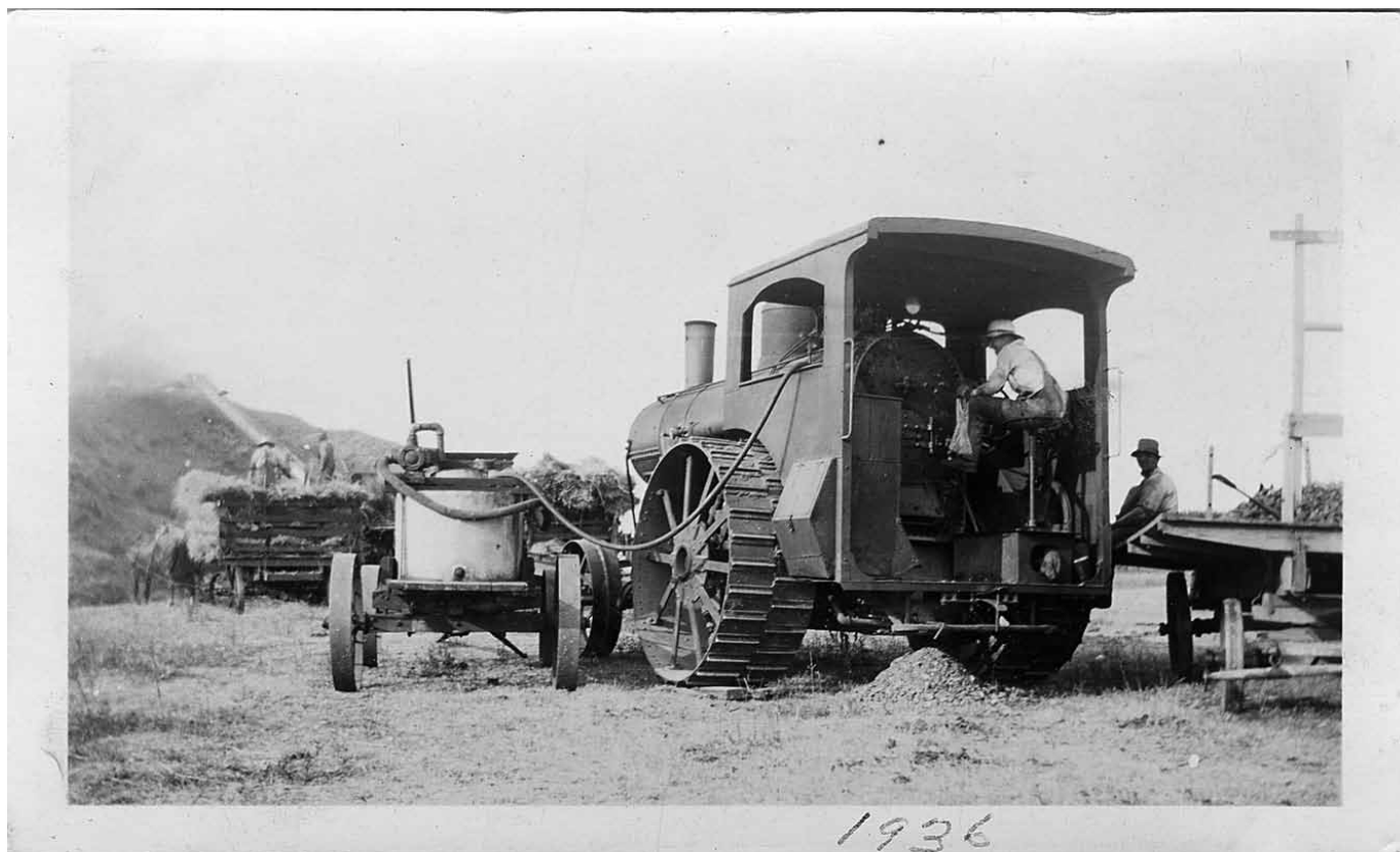
This was a steam tractor powering thresher on Stark Farm in DeKalb County. Power was transferred from the steam tractor to the thresher by a large belt, not visible in the photo. The thresher is operating in the background. Courtesy Illinois State Museum, photographer Robert Warren.
