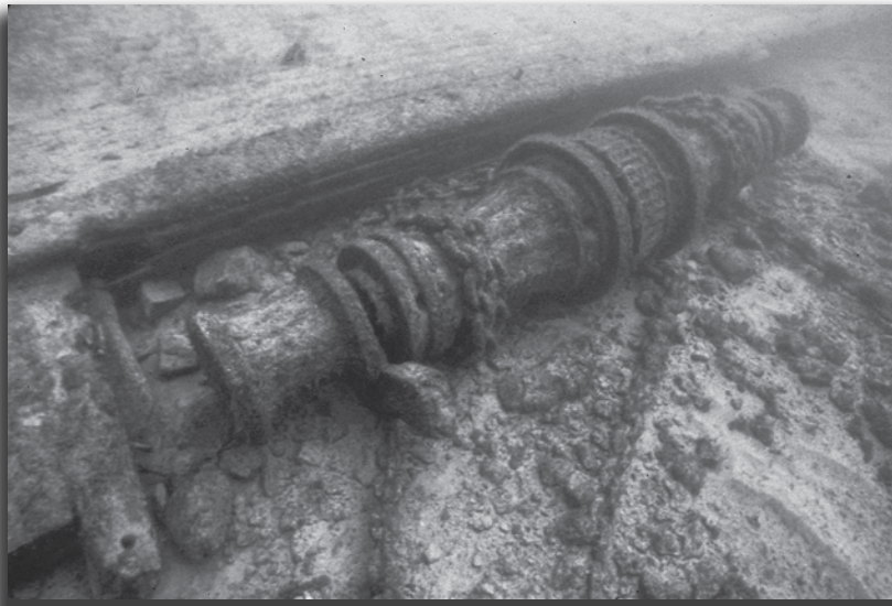
This is the windlass of the ill-fated 1860 steamer, the Lady Elgin. A windlass lifts a ship's anchor and chain. Photo by Claire Gadbois, Underwater Archaeological Society of Chicago.
